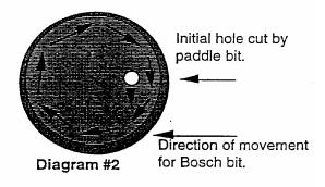
Insert the router in 3. the hole and move toward the edge in a clockwise direction.
